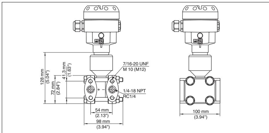
Fig. 61: DPT10, Conexão 1/4-18 NPT e RC 1/4
