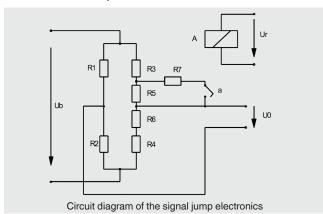
With these force transducers, four variable resistors (R1 ... R4) are connected together to form a Wheatstone bridge. When the measuring body deforms, the opposing resistors are stretched or compressed in the same way. This leads to a detuning of the bridge and a diagonal voltage U0.
