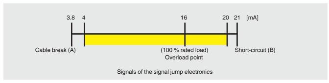
With a fixed signal jump of, for example, 4 mA, the test cycle can then be triggered, in any operating state, by activating the test relay. The upper measuring range limit of 20 mA will never be reached and thus the checking of the signal jump is enabled.
