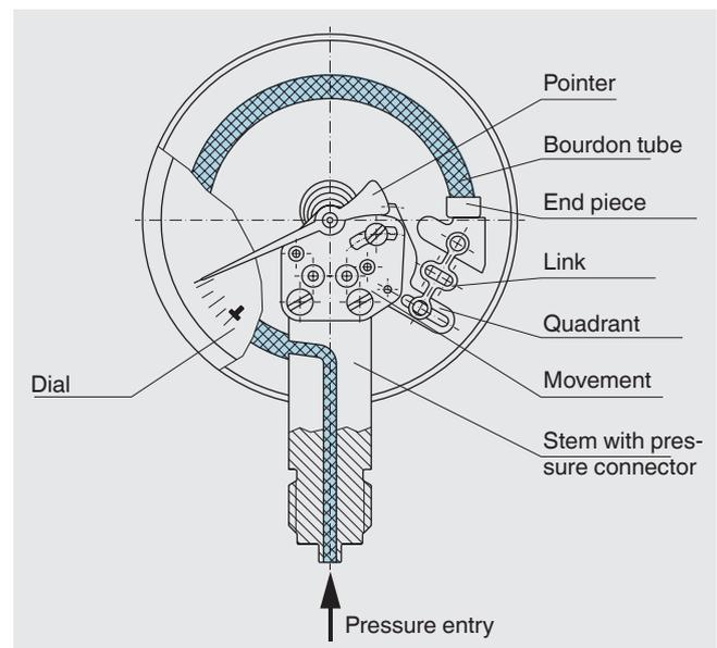
Fig. Pressure gauges with bourdon tube
