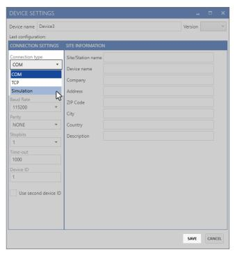
This device can now be used as if connected to a normal device; when connected to the simulation mode device it will play a default log file and simulate a FLC-UFL Series flow meter measuring flow.
